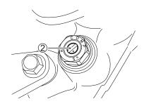
To set the compression damping force adjuster to the standard position, turn the adjuster clockwise until it stops and then turn it counterclockwise 8 clicks until the two punch marks align. If the two punch marks do not align by turning out 8 clicks, turn in or out the adjuster until two punch marks align.
