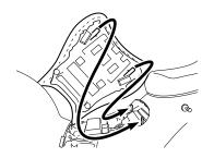
To reinstall the seat, slide the seat hooks into the seat hook retainers on the frame and tighten the bolts securely.
