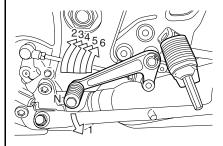
This motorcycle has a 6-speed transmission which operates as shown. To shift properly, squeeze the clutch lever and close the throttle at the same time you operate the gearshift lever. Lift the gearshift lever to upshift and depress the lever to downshift. Neutral is located between 1st and 2nd gear. When neutral is desired, depress or lift the lever halfway between 1st and 2nd gear.
