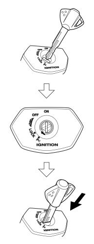
Align the lid hole position with the key hole position when inserting the key.
