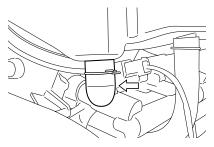
10.Remove the plug and drain water and oil at the periodic maintenance interval. The air cleaner drain plug is located beneath the air cleaner box.
