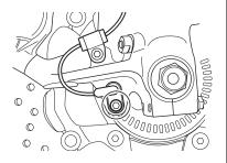
2. Remove the front wheel speed sensor by removing the mounting bolt.
