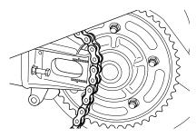
With the wheel moved forward, remove the chain from the sprocket.
