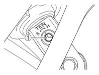
To set the rebound damping force adjuster to the standard position, turn the adjuster clockwise until it stops and then turn it counterclockwise 12 clicks until the two punch marks align. If the two punch marks do not align by turning out 12 clicks, turn in or out the adjuster until two punch marks align.
