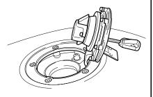
To open the fuel tank cap, insert the ignition key into the lock and turn it clockwise. With the key inserted, lift up with the key and open the fuel tank cap. To close the fuel tank cap, push the cap down firmly with the key in the cap lock.
