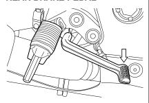
Depressing the rear brake pedal will apply the rear disk brake. The brake light will be illuminated when the rear brake is operated.
