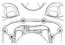
Remove the fasteners. Remove the under cover.
