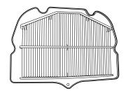
Inspect the air cleaner element condition. Replace the air cleaner element periodically.
