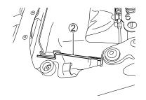
4. Remove the prop stay ② if the prop stay is equipped.
