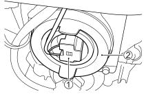
1. Disconnect the socket ① from the headlight and remove the rubber cap ②.
