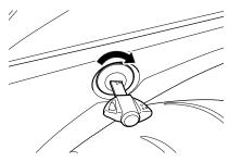
The seat lock is located under the left frame cover. To remove the rear seat, insert the ignition key into the lock and turn it clockwise.
