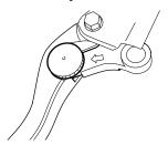
The distance between the grip and the clutch lever is adjustable to 4 positions. To change the position, push the clutch lever forward and turn the adjuster to the desired position. When changing the clutch lever position, always be sure the adjuster stops in the proper position; a projection of the clutch lever pivot should fit into the depression of the adjuster. This motorcycle is delivered from the factory with its adjuster set on position 2.
