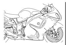
6. Remove the bolts and hooks of the right fairing ④.
