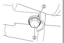
3. Remove the drain plug ② and gasket ③ from the bottom of the engine and drain the engine oil into a drain pan.
