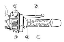
Suzuki Drive Mode Selector 4 Engine power characteristics can be selected from 3 modes by operating the drive mode selector to suit rider's preference in various riding conditions.
