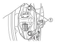
3. Remove both brake calipers from the front forks by removing 2 mounting bolts ① on each of the calipers.
