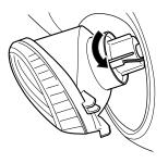
2. Turn the socket counterclockwise and remove it.
