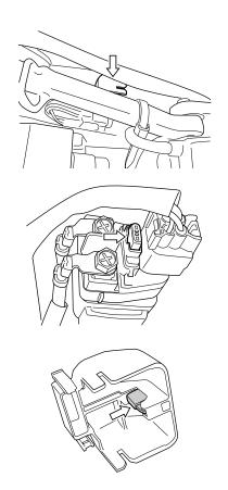
The main fuse is located under the front seat. To access the fuse, remove the seat by referring to the SEAT LOCK AND HELMET HOLDERS section. One 30A spare fuse is located inside the fuse box cover.
