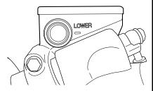
The clutch release mechanism of this motorcycle is operated by hydraulic pressure. There is no adjustment needed on the clutch release system because the system is self adjusting. However, inspect the following each time before driving to make sure that the system is in good condition and functioning properly.
