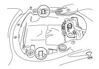
This motorcycle has helmet holders under the rear seat. Hook your helmet on the helmet holder and lock the seat.
