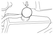
Remove the filler cap and add specified engine coolant through the filler hole until it reaches the "F" line. Refer to the FUEL, ENGINE OIL AND COOLANT RECOMMENDA-TIONS section.
