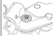
To set the rebound damping force adjuster to the standard position, turn the adjuster clockwise until it stops and then turn it counterclockwise 8 clicks.
