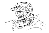
To reinstall the seat, slide the seat hooks into the seat hook retainers and push down firmly until the seat snaps into the locked position.
