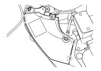
2. Remove the bolt and screw. Remove the upper right and left panel by unhooking the hooks.
