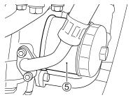
7. Turn the oil filter ⑤ counterclockwise and remove it with a Suzuki "cap type" oil filter wrench or a "strap type" filter wrench of the proper size.
