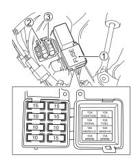
The fuses are located behind the upper left panel under the left handlebar. Remove the upper left panel by referring to the FRONT TURN SIGNAL LIGHT section.
