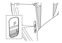
The engine coolant solution should be between the "F" (full) and the "L" (low) level lines on the engine coolant reservoir. If the level is lower than the "L" level line, bring it up to the "F" level by adding specified engine coolant.
