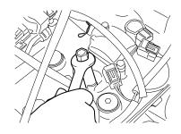
9. Remove the spark plug with a spark plug wrench.
