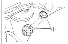
3. Remove the fuel tank fitting bolts ①.
