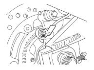
Remove the rear wheel speed sensor by removing the mounting bolt.
