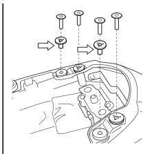
Install the attached washer and tighten the removed 4 bolts to the specified torque.
