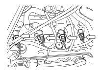
7. Release the coupler locks and disconnect the couplers from the ignition coils.
