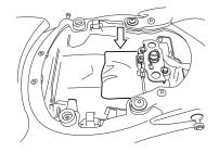
A tool kit is provided with your motorcycle. It is located under the rear seat.
