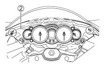
2. Remove the fasteners. Remove the upper meter panel ② by unhooking the hooks.
