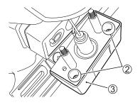
Remove the screws ② and take off the cover with the lens ③.
