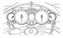
3. Remove the bolts. Unhook the hooks to lift the instrument panel ③.
