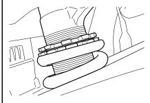
The adjustment can be performed by changing the adjuster ring position. However, Suzuki recommends that this adjustment be done by your authorized Suzuki dealer, since a special tool is needed for this job.
