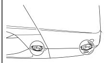
5. Remove the fasteners.
