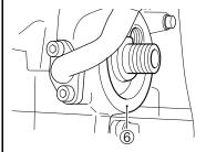
8. Wipe off the mounting surface 6 on the engine where the new filter will be seated with a clean rag.
