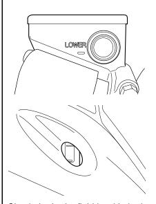
Check the brake fluid level in both the front and rear brake fluid reservoirs. If the level in either reservoir is below the lower mark, inspect for brake pad wear and leaks.
