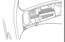
The frame number ① is stamped on the steering head as shown in the illustration. The engine serial number ② is stamped on the crankcase assembly.
