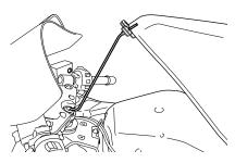
Lift the front end of the fuel tank and prop it up as shown above. Insert the crank end of the prop stay into the hole of the steering shaft.
