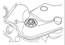
To set the spring pre-load to the standard position, turn the adjuster ① clockwise until it stops and then turn it counterclockwise 6 turns
