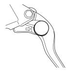
The distance between the throttle grip and the front brake lever is adjustable to 5 positions. To change the position, push the brake lever forward and turn the adjuster to the desired position. When changing the brake lever position, always be sure the adjuster stops in the proper position; a projection of the brake lever pivot should fit into the depression of the adjuster. This motorcycle is delivered from the factory with its adjuster set on position 3.
