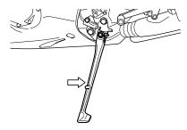
An interlock system is provided to cut off the ignition circuit when the side stand is down and the transmission is in any gear other than neutral.
