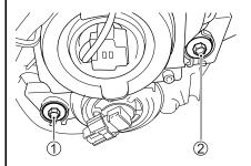
**To adjust the beam up and down:** Turn the adjuster ① clockwise or counterclockwise.
