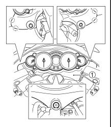
Remove the bolt and fasteners. Remove the lower meter panel ① by unhooking the hooks.
