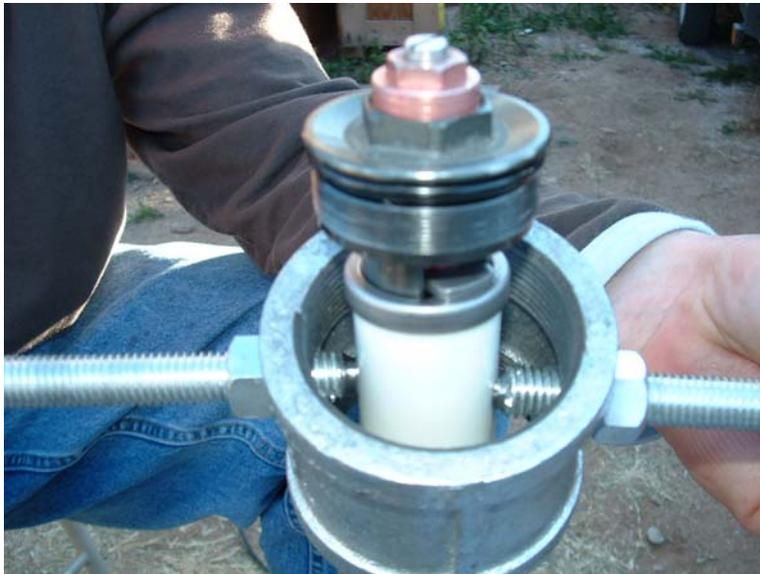
**Lift the upper fork tube up, and tighten the fork nut to the upper tube. Congrats your done!
