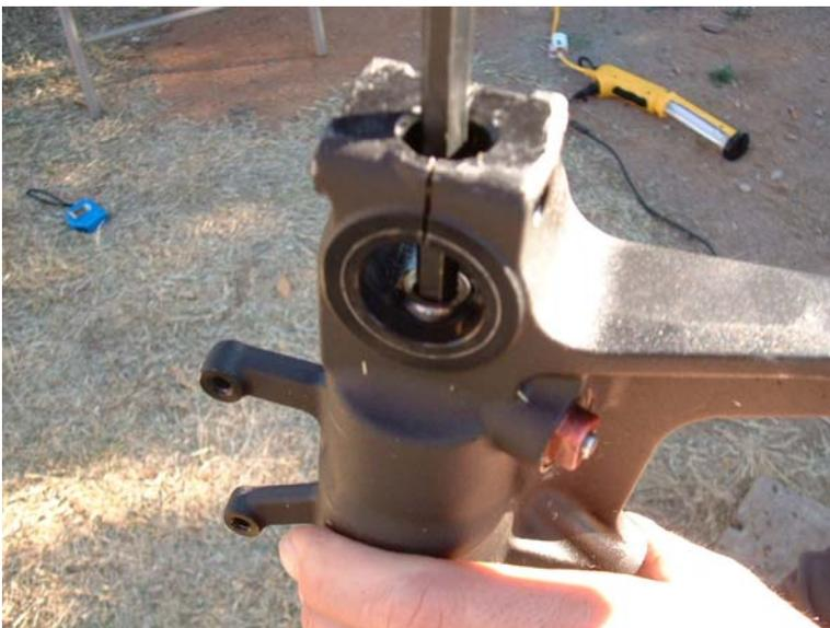
**Pull the cartridge out and pump to remove all oil.**
