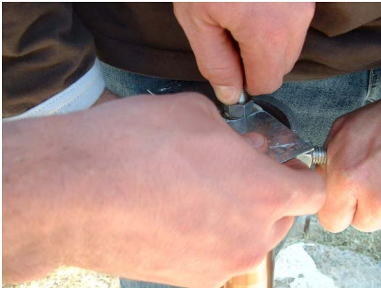
**Spring compressed and spacer-jam removed, carefully lift the compressor up and remove the spacer.**
