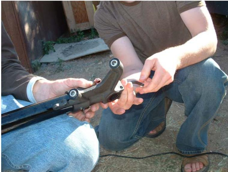
**Hold the rod up for easier filling. Start out with about a 1/4 qt. Then pump the cartridge, it will drop level quickly as the air is removed from inside the cartridge.**
