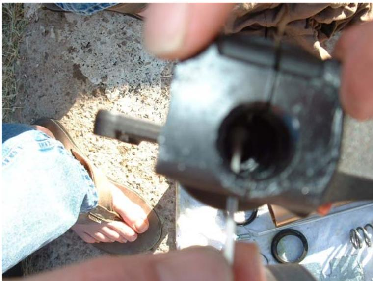
**Insert cartridge, and press the top over to one side. Locktite the bolt, insert in bottom of lower tube, and tighten to spec.**
