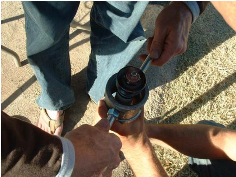
Have your assistant hold the fork tube steady, while you compress the spring. Once compressed your assistant needs to slide the spacer-jam over the spacer and below the jam-nut. This will capture the spring in a compressed state, allowing access to hold the jam-nut so you can unscrew the fork nut.
