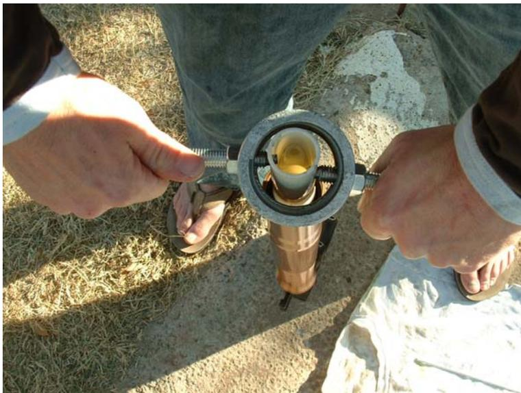
Next pull the spring out. \*NOTE\* on the Busa there will be a small metal cup on top of the spring, make sure you check how it is placed on the spring.
