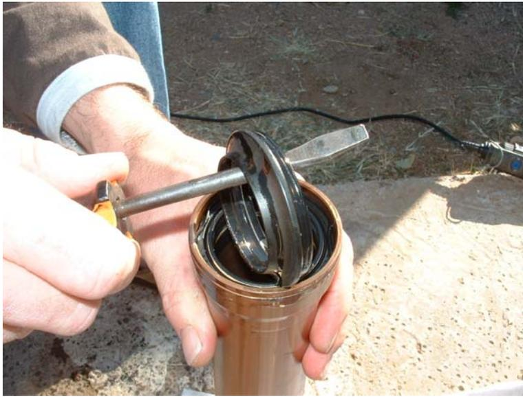
**Remove the Seal retainer spring. Simply pull one side out, and rotate around, it is a split ring fitted into a groove.**
