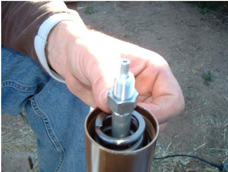
**Grab the spacer and compressor, place over the fork springs, and compress once again, and slip the spacer-jam into position. Before you compress, lift the rod to the fullest extended position, it will sink slowly as your compressing, so work quick. If its too low to get the jam plate in, thread fork nut onto rod and lift the rod while compressing spring.**
