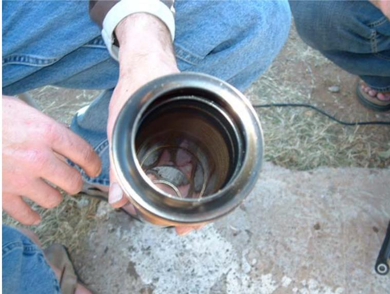
**Carefully slide upper tube over lower tube, and work its way down to the fully seated position. If there is any resistance you may have a bent fork (this was the case on this particular fork set).**
