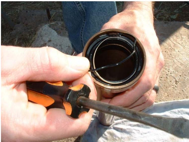
Carefully pry the seal out, again, dont scratch the inner tube area.
