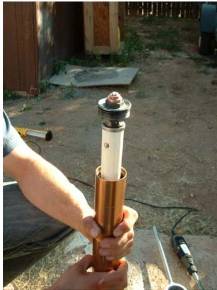
**Slip your fork spring compressor you just made over the fork nut, thread the rods so the ground down end is inside the hole of the spacer (white plastic tube, but on the Busa its aluminum).**
