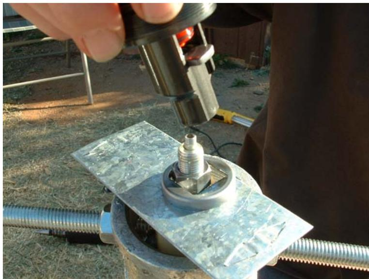
**Remove the Rebound Adjustment Rod, simply pull up, watch out there is oil inside it.**
