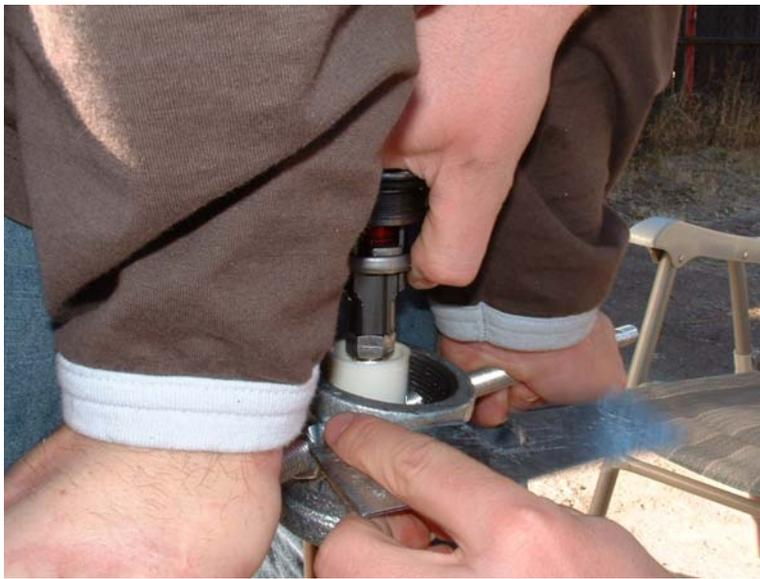
**Sliding the spacer-jam into position, again, below the jamnut and above the spacer.**
