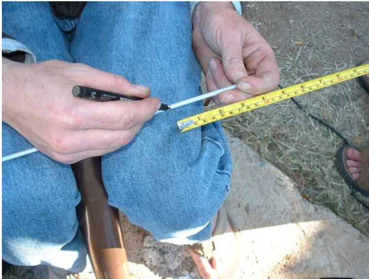
Hold rod inside tube, and the bottom of the rod should barely touch the end of the rod when the mark is level with the top of the tubes.
