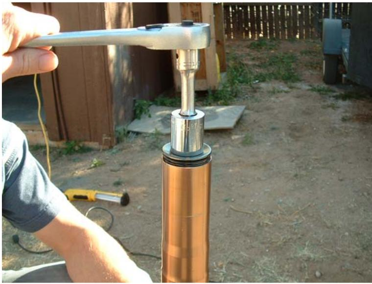
**Slide the upper fork tube down to the bottom position.**
