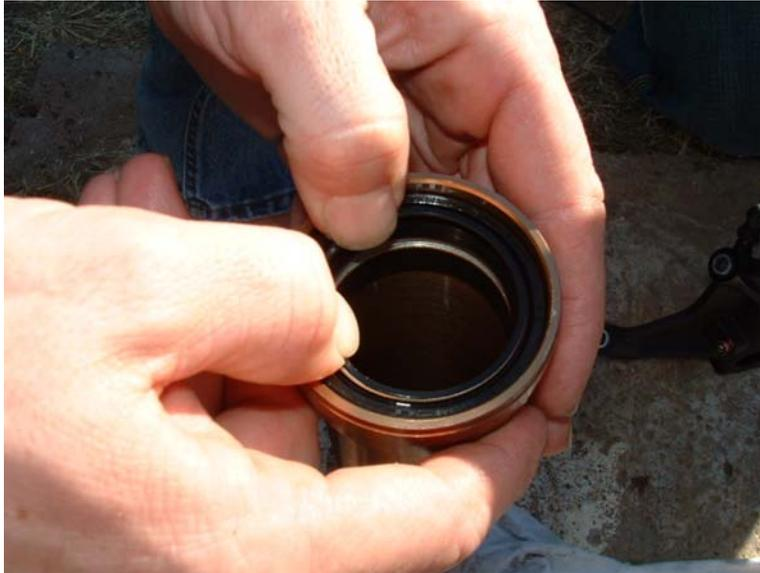
**Install seal retaining ring, press it into the groove and work it around. If its not in the groove the seal is not fully seated.**
