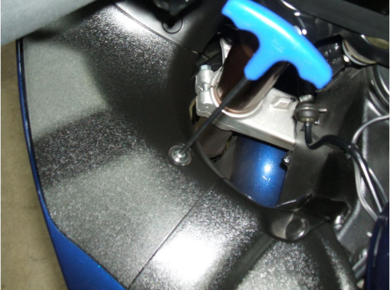
2<sup>nd</sup> Step Remove these plastic pin (both side) by inserting a small flat head screw driver and popping it up.
