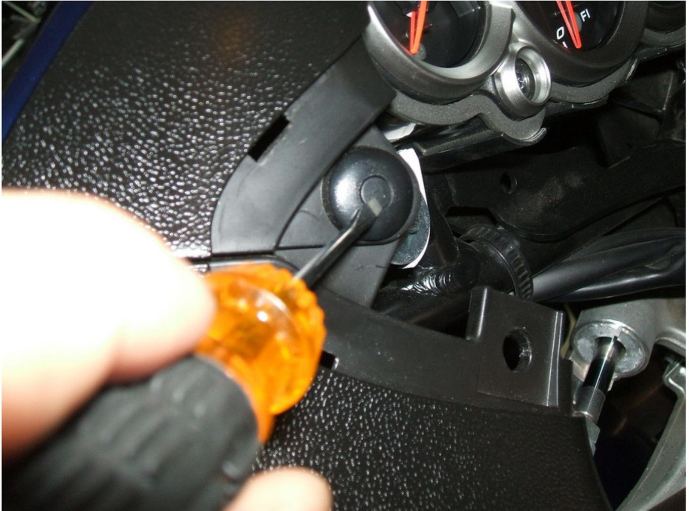
Step 6: Small pin on the upper corner of the trim piece. Push in center to remove (Both Sides)
