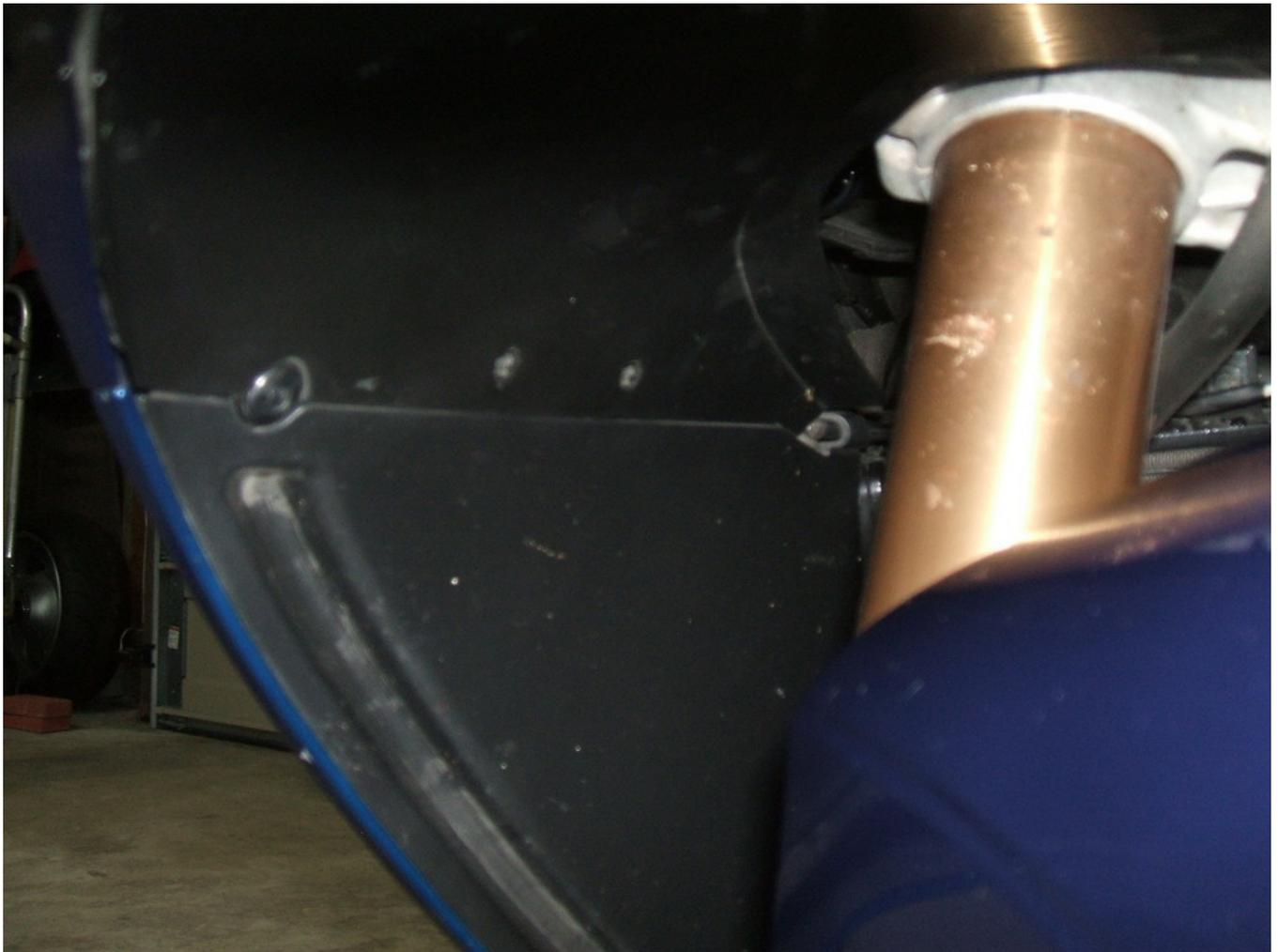
Step 14: Taking out the Gauge Cluster. Two bolts, 8mm, on both sides. Be careful pulling the gauge out. Behind this bolt there is a washer.
