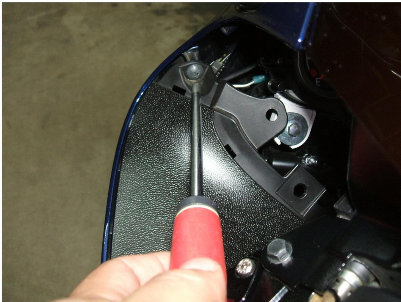
Step 9: See the Fuse Block?! Now if you need to remove the Upper Cowl, you will need to remove this screw.
