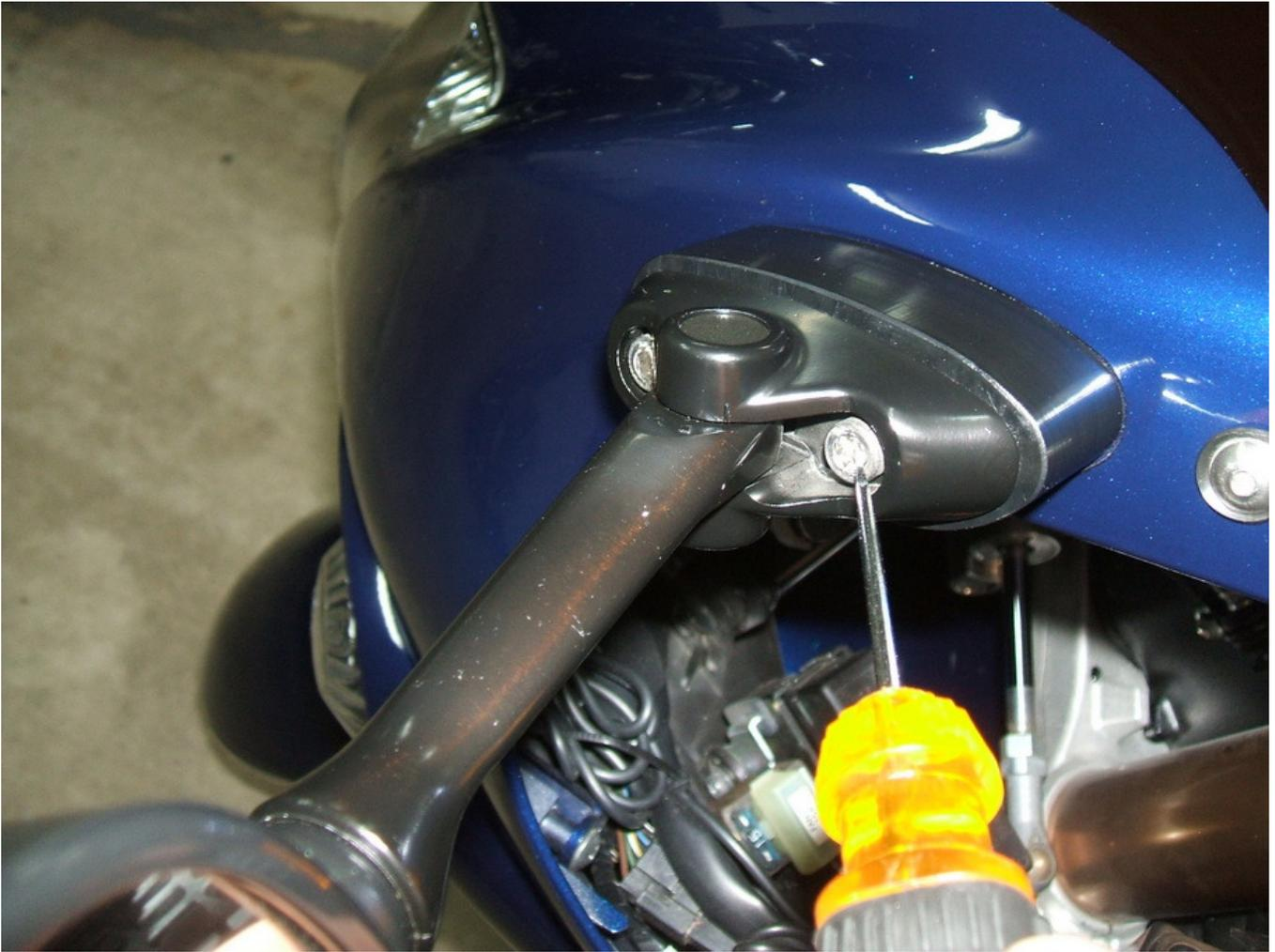
Step 13: There will be 6 small push pins that needs to be removed. Here are the front two.
