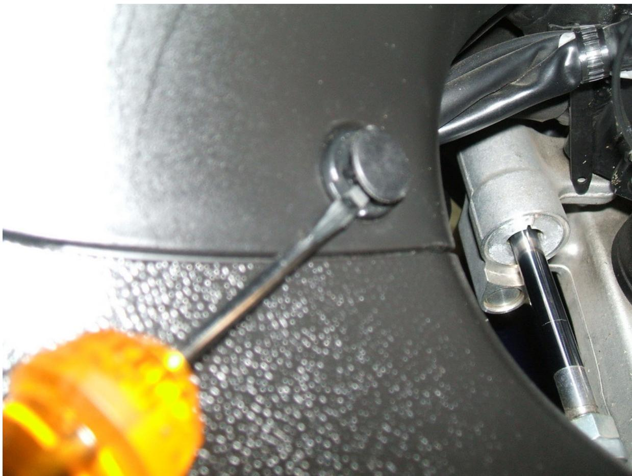
Step 3: Remove this bolt located center and below the triple Tree.
