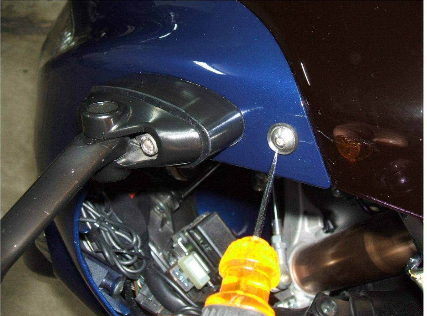
Step 12: Remove the mirror mounts Yes you have to... its attached to the upper cowl frame.
