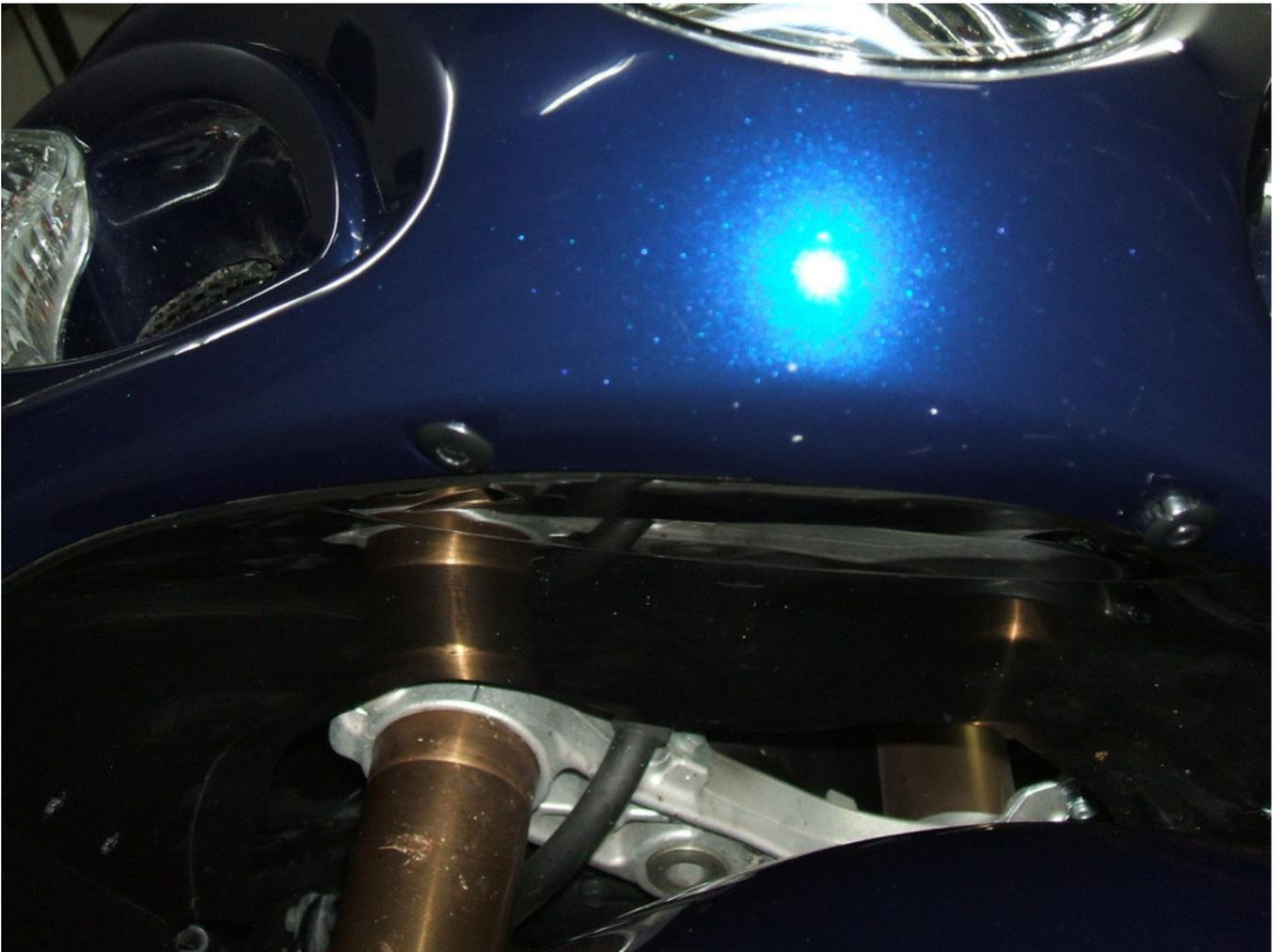
Two more on each sides of the fairing. Note: The far pin cannot be seen here. See Blanca's Fairing removal!
