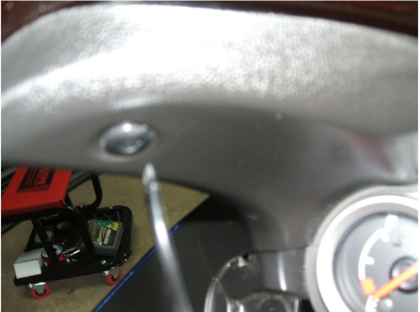
Step 7: Now this is where people panic! The upper trim piece is very tightly fitted. You can either use a flat head screw driver to separate this trim piece with the other plastic piece of the cowl and pull outward. Or just pull one corner of the trim until it pops out and do the other corner. Gut wrenching plastic cracking noise. It's ok!
